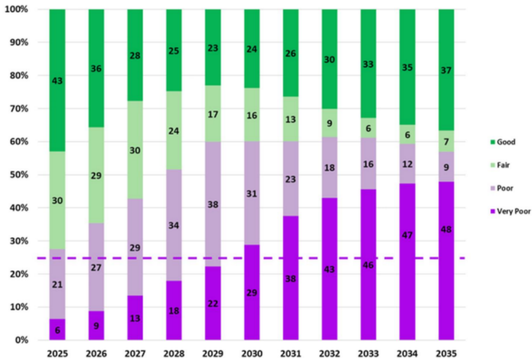
Forecasted Pavement Condition Distribution with an Annual Investment of $103 Million
