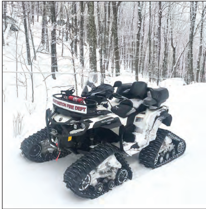
Huntington Fire and Rescue's tracked rescue ATV, which allows another unique aspect of the service the Department is able to provide for calls in the high mountains and backwoods.
